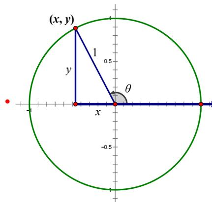
trigonometry being careful to note the signs of  $x$  and  $y$ . In the figure as drawn in the second quadrant, for example,  $x$  is negative and  $y$  is positive, which implies that  $\sin \theta$  is positive and  $\cos \theta$  and  $\tan \theta$  are both negative.
